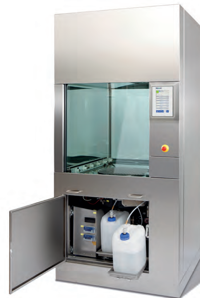
Accommodation of 2 10 l containers below the machine. The containers can be separately removed, enabling highly ergonomic replacement.
