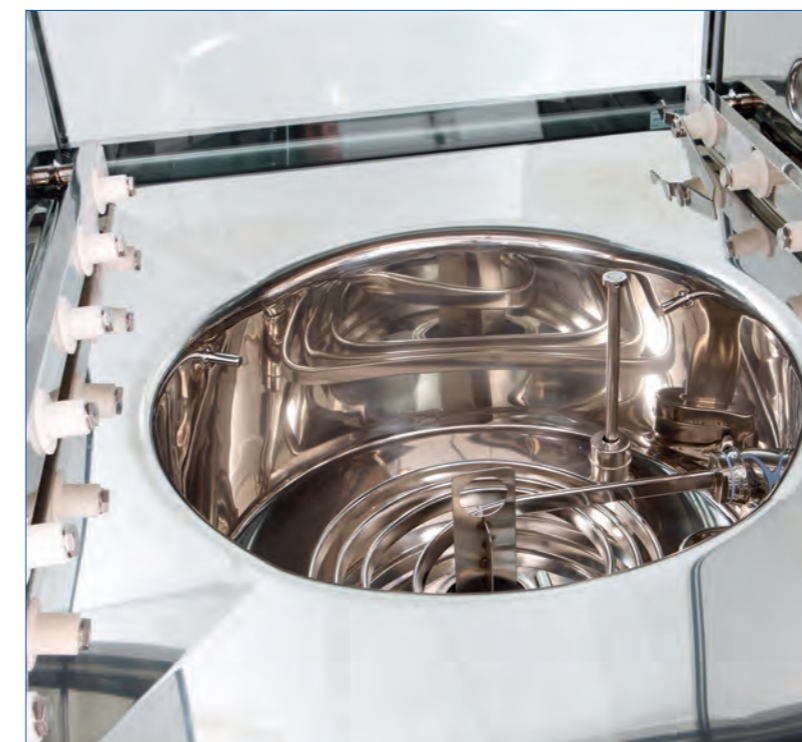
Washing tank made of mirror-finished sheet metal with installed heating elements and fine screen in the pump suction pipe.
