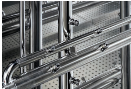
Multiple horizontally and vertically mounted oscillating arms equipped with stainless steel spraying nozzles.
