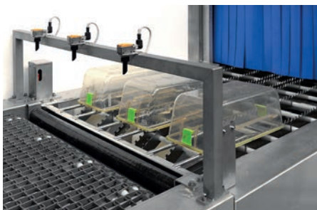
Cage inverter is equipped with a photo-cell positioning sensor
