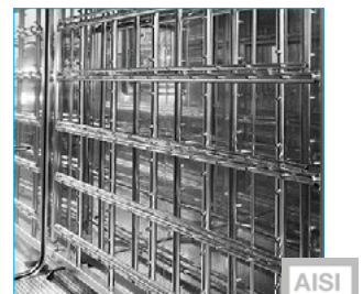
Washing chamber made of s.s. AISI 316L
