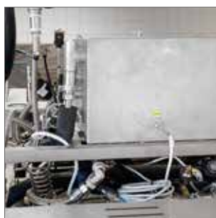
A built in degassing device placed on top of the sterilizer allows the reduction of the NCG concentration of the water for steam generation below the 3,5% Vol. according to EN 285 norm.
